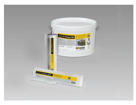
Aqueous-based intumescent product, white, pH neutral and solvent free. When a duct passes through a wall, it is applied to create a flame-retardant seal in the gap between the wall and the duct.
